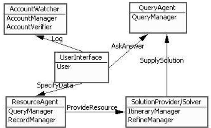
Figure 1: PIPS agent class diagram (extracted from the PIPS design documentation produced by Yenty Frily using agentTool)
